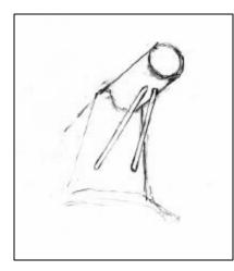
The next step in its evolution was the use of a dual support configuration, aimed at not only improving aesthetics, but distributing forces over a larger area across the base. Challenges presented by this iteration are the interface between the pedestal and base, and
