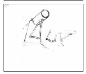
To alleviate the continued point – load concern, another strategy is to utilize a continuous steel rod formed to create a "saddle" of sorts, wrapping around the side of the pedestal. The ends could elegantly terminate in a parallel fashion and welded to the underside of the steel tube. For aesthetic reasons, welds could be made on the underside of the "saddle",
